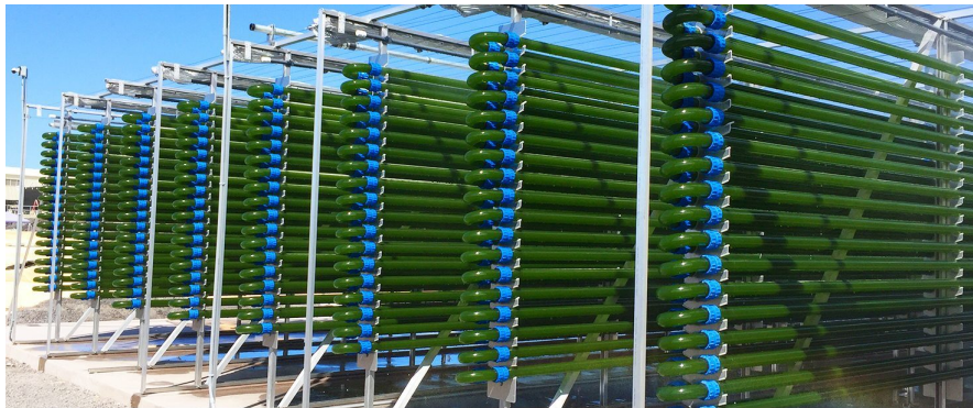
Figure: Tubular reactor
