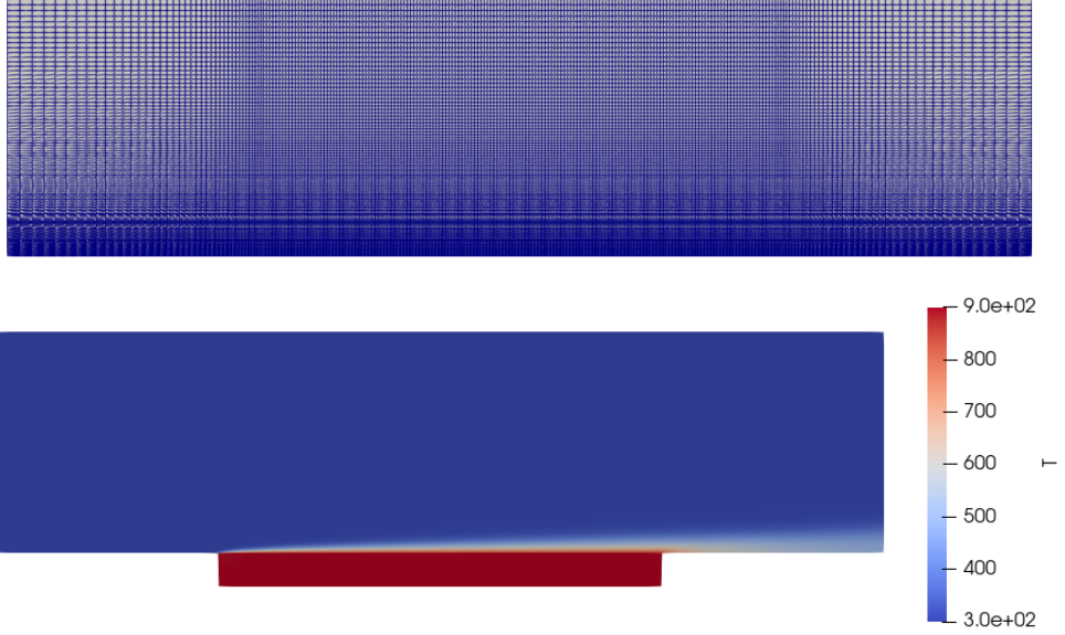
FIG. 6. Diagram of the FSI test case, consisting of a hot steel plate cooled by a cold air stream.
